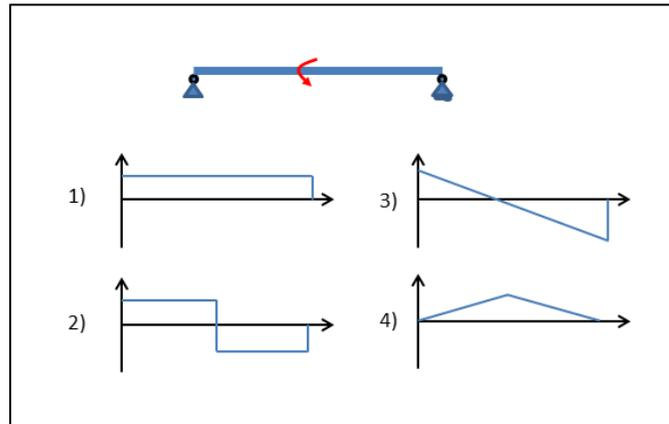
Figure 3 A typical quiz question, in this case testing understanding of the shear force distribution in a beam with a point moment applied.
