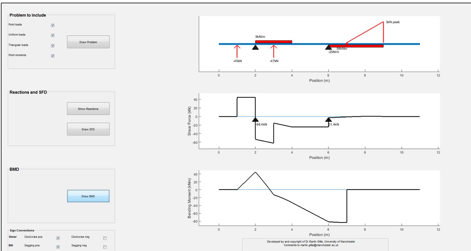
Figure 4 Screen-shot of the software developed for practicing calculating reaction forces, shear force diagrams and bending moment diagrams.
